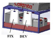
"air tight" bag system. To drain the tanks after use the operator simply positions a bag on the lower frame and opens a tap, the tank solution then under gravity, runs quickly into the bag until the tank is empty. To refill the tank again the operator moves the bag to a position above the processor tank and opens the tap and under gravity the chemical flows back into the tank. A clean and easy system with no expensive and troublesome pumps used.
